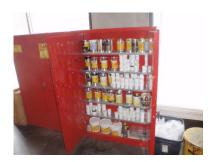
**Proper** storage of flammable liquids in a designated and properly designed cabinet.
